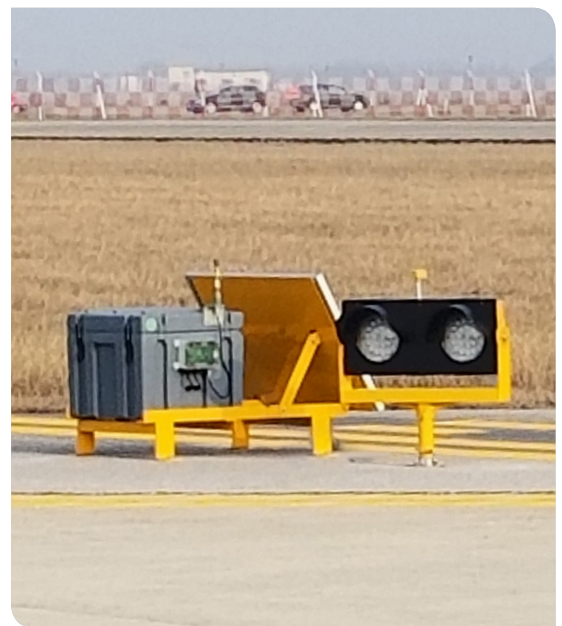
Avlite's ERGLs (above) enhance safety at critical runway intersections for the F-16 fighter squadrons at Aviano Air Force base.
