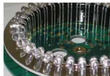
LEDs are able to be arranged in rows, rings and clusters
